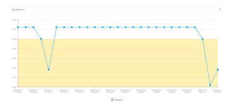
Remote monitoring of battery voltage levels with low, dead low and ultra-high voltage alarms
